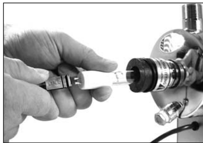
Step 4 & 5 - Remove Sockets
